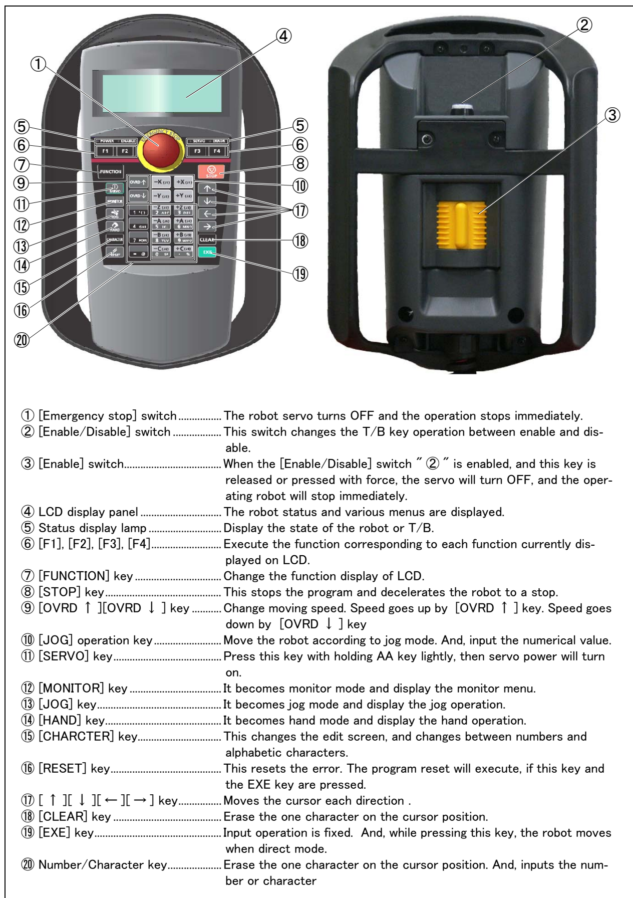
Fig.3-30 : Teaching pendant key layout and main functions
